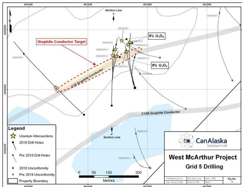
The unconformity-related uranium mineralization intersected in Cameco’s discovery holes, WMA042 and WMA042-2, has been extended 50 metres to the south and at least 200 metres to the west.
